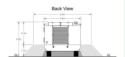
isolated earthing MV (earthing cable of MV trench) 000000 GL mineral grain mixture or recycling material 0/16, compacted and levellied
